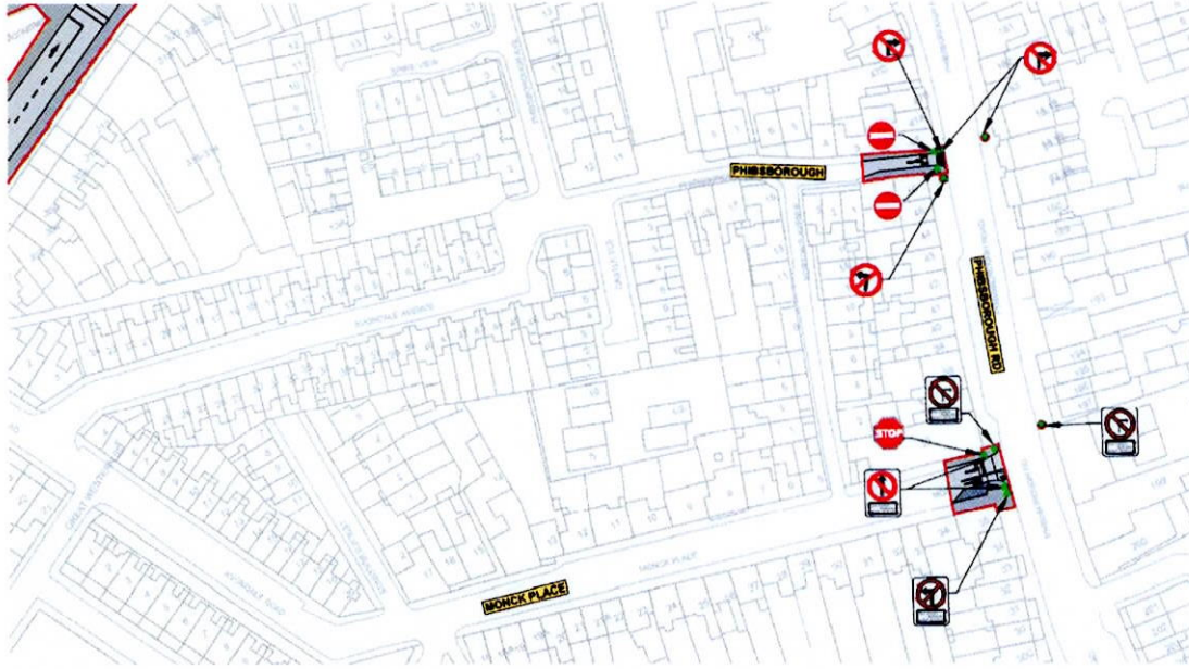
Extract of Bus Connects Plan to restrict traffic flow at Phibsborough Road, Monck Place & Avondale Avenue ('Phibsborough')
